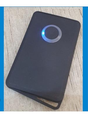
**UHF Scanner RE40** is a powerful RFID reader, capable of reading UHF tags and transmitting the acquired data to any device equipped with a Bluetooth interface, including Android or iOS smartphones and tablets.
