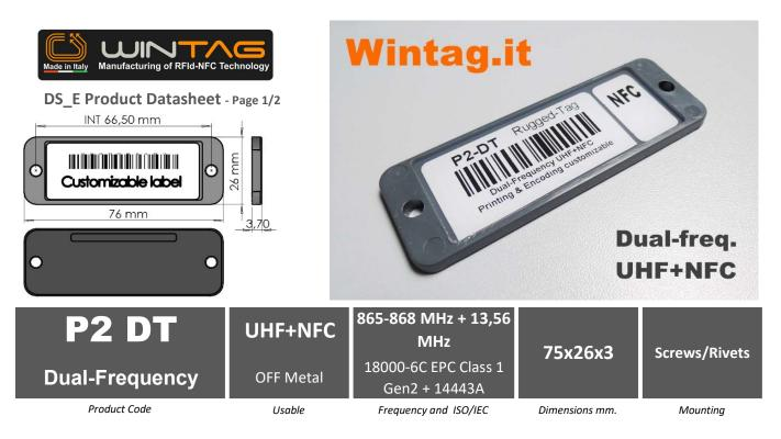
Dual-Frequency RFID tag, P2 Series, can be fixed with screws / rivets. RFID transponder UHF + NFC dualfrequency, made of very resistant rigid plastic, available in different versions, OFF Metal use. Inside there are 2 distinct UHF + NFC tags that can have the same electronic coding
