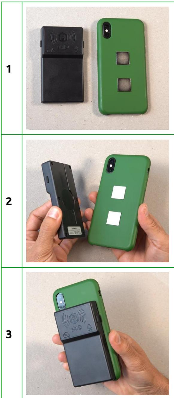
Fig. 1.10: Installation Notice - Magnets
