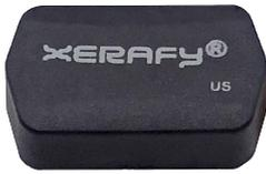
The Xerafy Pico Plus relies on high-performance engineered polymer to offer the smallest and most rugged RFID on-metal tag to industrial applications where critical and potentially hazardous situations require reliable identification of assets. The IP68 rated tag achieves stunning read ranges and can be attached to hand tools, equipments and medical devices.
