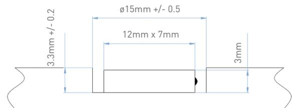
To properly embed PICO In, first prepare a socket to meet the dimensions shown in the socket dimension figure above.
