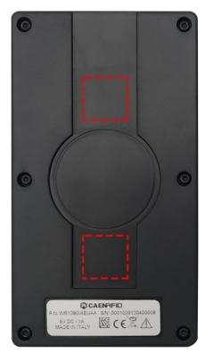
Fig. 1.9: Magnets Position
