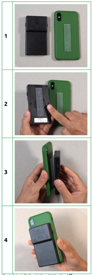
Fig. 1.12: Installation Notice - 3M Dual Lock™
