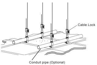
Run the Cable Wires through the Pipe Clamps.
